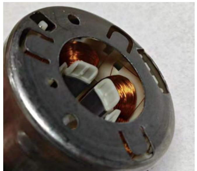
Figure 1: Schematic diagram of winding, iron core, and metal frame structure
